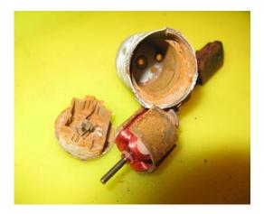
Pictures show corrosion on the inside of the motor.
